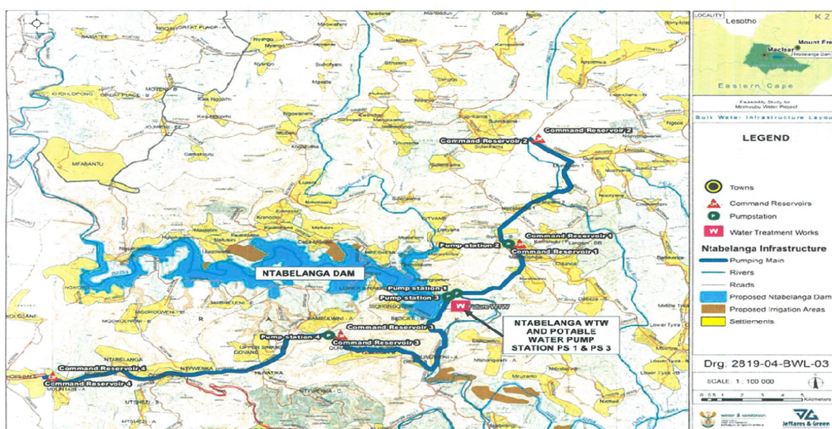
Figure 9-7: Primary Bulk Potable Water Pipelines, Pumping Stations and Command Reservoirs
